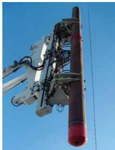
**The Herrenknecht Vertical box-on-box rig**, a containerized rig with cylinder hoisting system for drilling in urban areas for geothermal as well as oil and gas. The rig has a box-on-box substructure and a threesectioned mast that is foldable in width, fulfilling stan-
