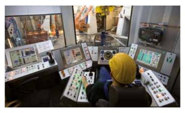
Modern driller's cabin to control rig and pipe handling operations
