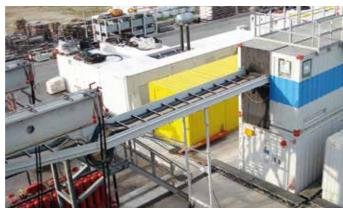
**Integrated extension system** between rig and backyard for easy and fast **skidding without disconnection** of hoses and cables
